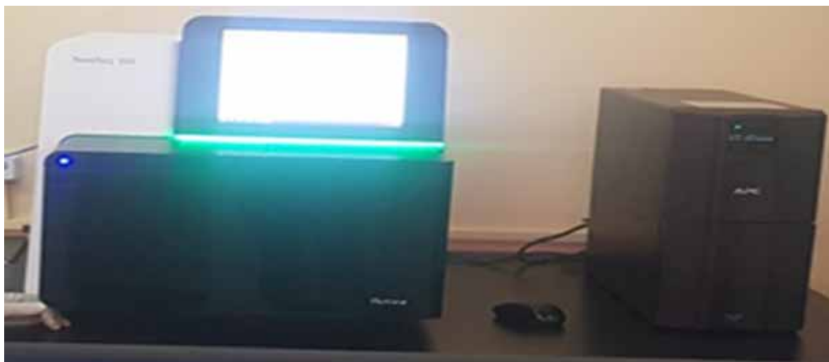
Figure 8: Next Generation Sequencer (NGS), Illumina Next Seq 550
