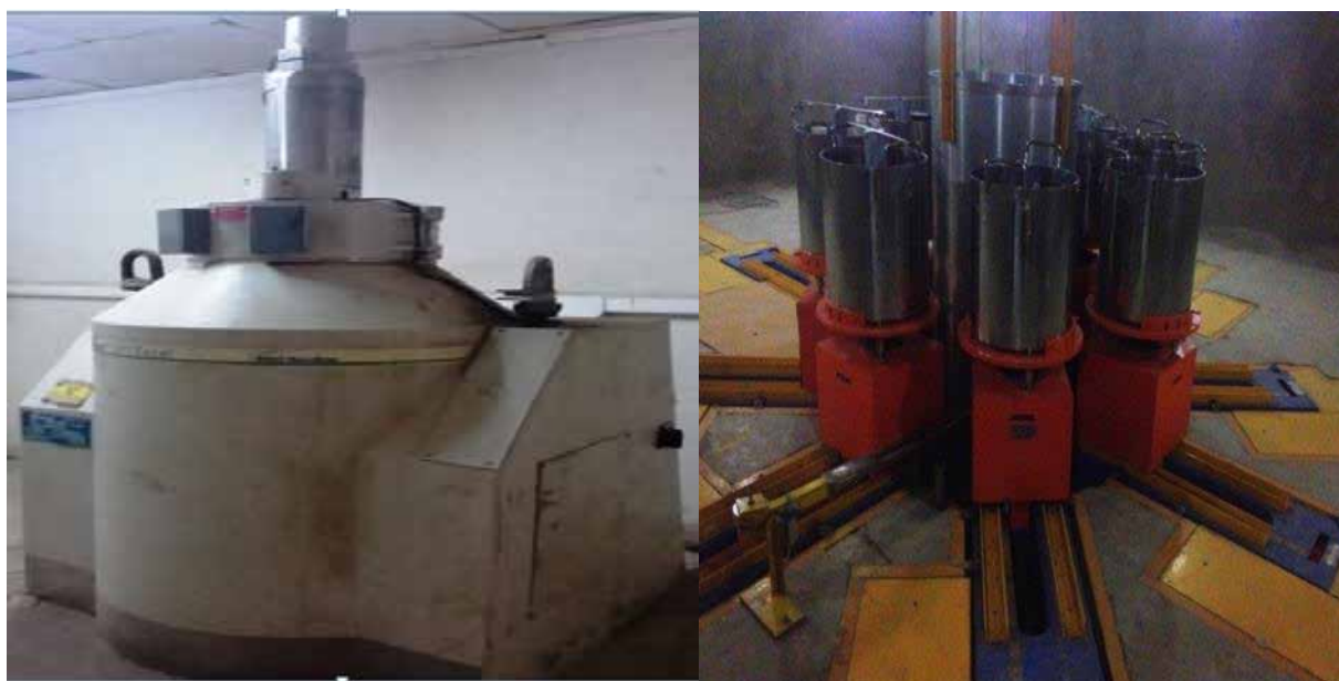
Figure 11: Cobalt 60 Dry cell radiator
